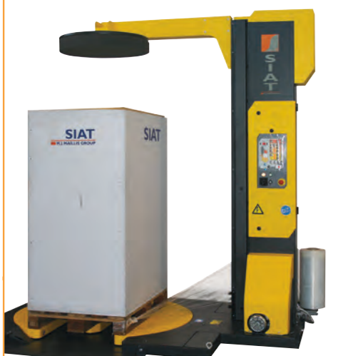
Pressing unit for unstable pallet available for all models
